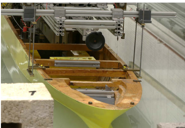
Figure 15. Mechanical safety device to protect the ship model from touching the bottom.
