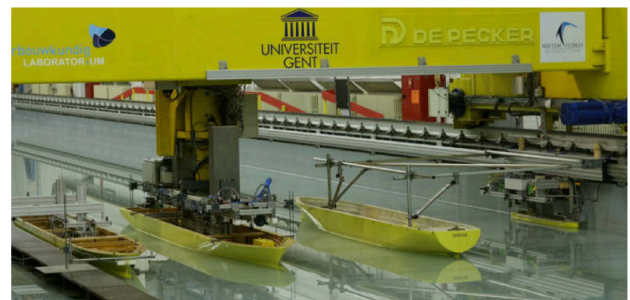
Figure 10. Auxiliary carriage for ship interaction tests.
