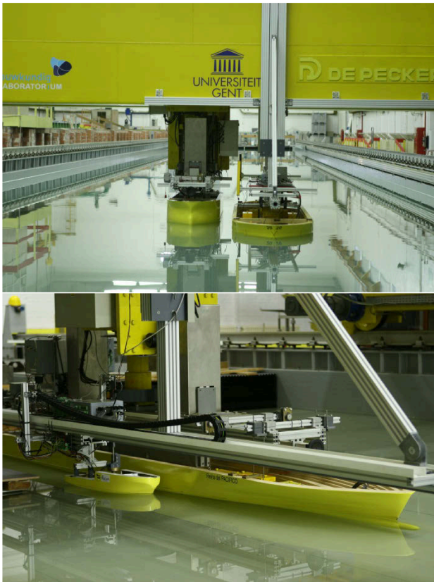
Figure 11. Second beam for the execution of ship - ship interaction (top: lightering operation between VLCC and Aframax tankers [3]; bottom: ship - tug interaction)
