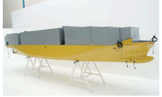
Figure 1. A model of the large container ship with twin propellers and rudders
