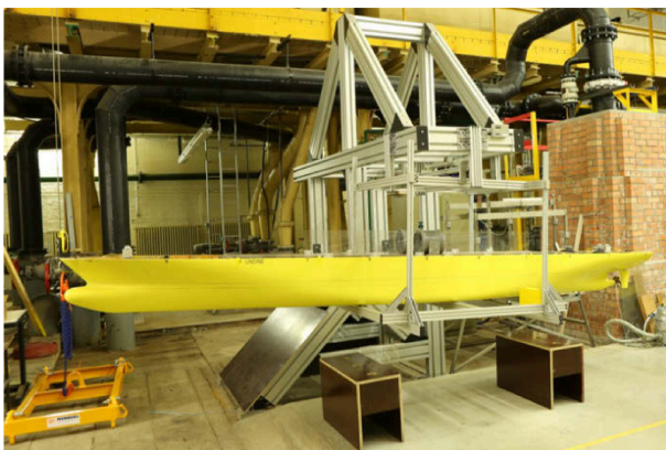
Figure 8. Determination of the moments of inertia (principle of the physical pendulum).
