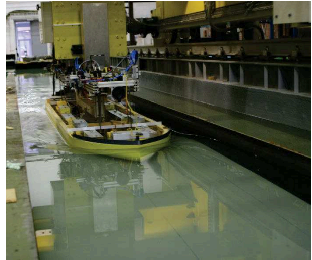
Figure 2. KVLCC2 model during an experiment.
