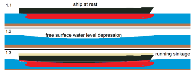
Figure 1. Ship and water at rest (1.1), return flow induced free surface water level depression (1.2), the sailing ship displacing the same volume of water as in 1.1 but having less under keel clearance (1.3).
