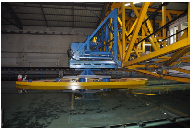
Figure 4. HPMM device and model ship on the false-bottom.
