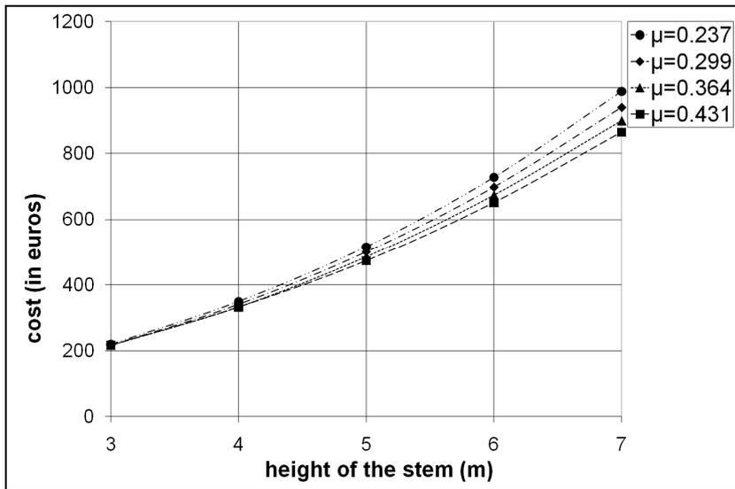
Figure 3. Cost variation for different base friction angle
