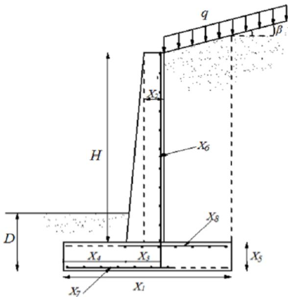
Figure 1. Cross section of the RCC retaining wall.
