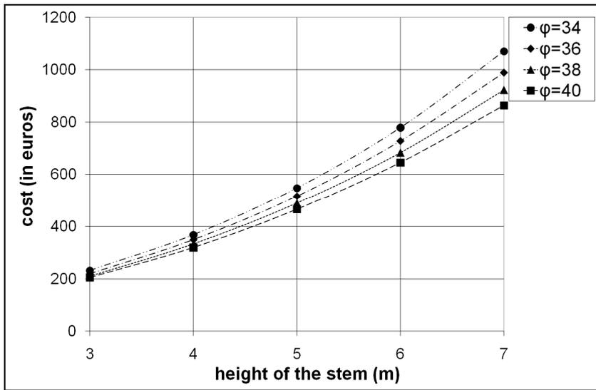
Figure 4. Cost variation for different backfills
