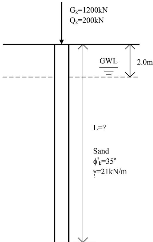
Figure 1. Pile foundation example (after Orr 2005a).
