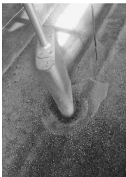
Figure 10. Photograph showing scour around round nosed pier
