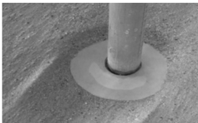
Figure 2. Photograph showing scour around the pier fitted with collar
