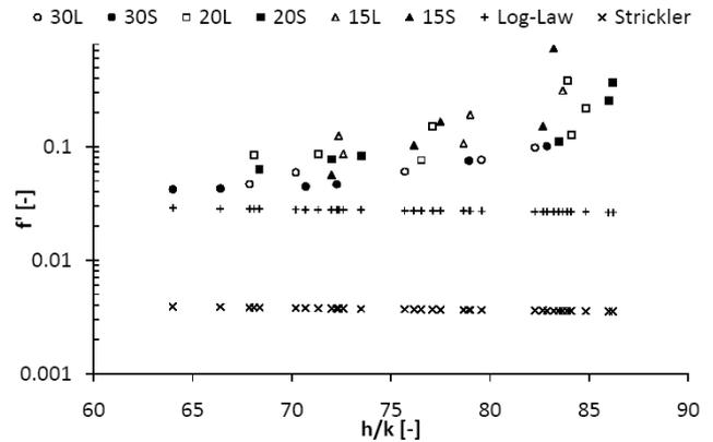
Figure 7 Observed and calculated surface friction as a function of relative submergence.
