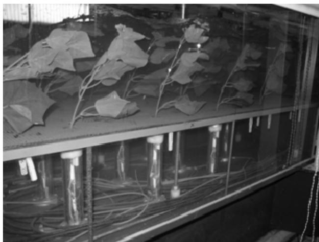
Figure 1: Setup of DFS test section and artificial poplars under flow action.
