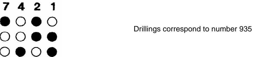
Fig. 4 a – d: Examples of combinations of numbers by arrangement of drilling holes. The numbers will be „read“ by using a template.
