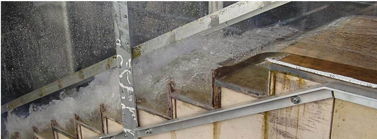
Figure 3. Transition flow regime on porous pooled stepped spillway ( Po = 5\% ): d_c/h = 0.51 ; q_w = 0.036 \text{ m}^2/\text{s} ; Re = 1.4 \times 10^5
