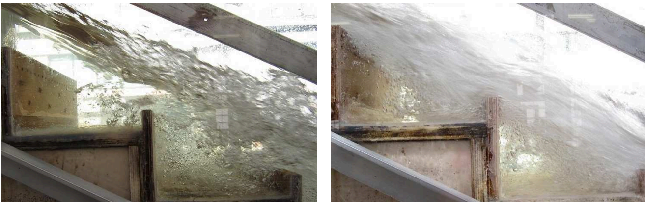
Figure 4. Cavity detail and flow through pores in skimming flow regime on porous pooled stepped spillways – Left: Po = 5\% , d_c/h = 1.44 ; q_w = 0.171 \text{ m}^2/\text{s} ; Re = 6.8 \times 10^5 ; Right: Po = 31\% , d_c/h = 0.86 ; q_w = 0.079 \text{ m}^2/\text{s} ; Re = 3.1 \times 10^5
