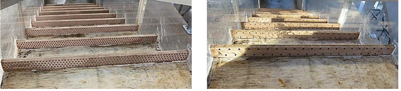
Figure 2. Photos of porous pooled stepped spillways with Po = 31\% (Left) and Po = 5\% (Right); Diameter of holes \varnothing = 5 mm
