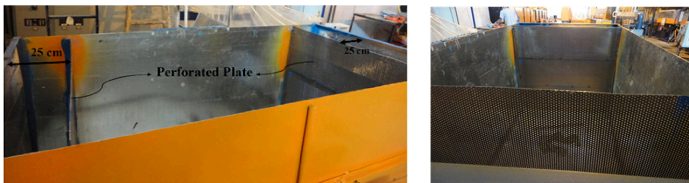
Figure 1. A view of the rectangular cube and installation of the perforated plates
