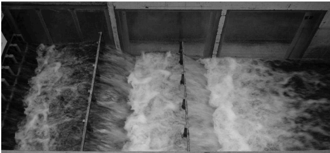
Figure 9. Nappe flow conditions in the pooled step cascade scale model (scale 1:12) for FCA-CRT Kruibeke, corresponding to a water level of +6.8 m TAW in the river Scheldt
