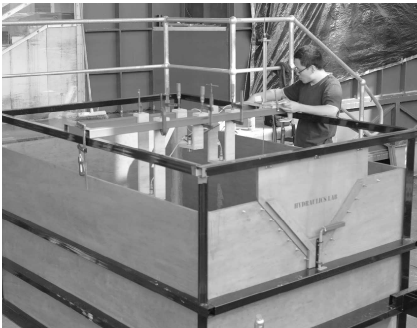
Figure 2. Reservoir and V-notch overflow, with the V-notch overflow gate closed (foreground right) - The displacement meters are mounted above the reservoir
