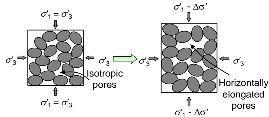
Under the same shear stress ratio,  $i_{start}$  increases with confining stress
