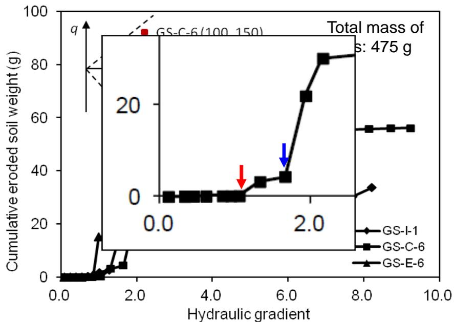
Cumulative eroded soil mass
