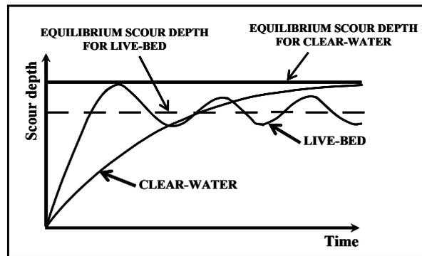
Figure 1. Scouring in clear-water and live-bed conditions (Raudkivi, 1998).
