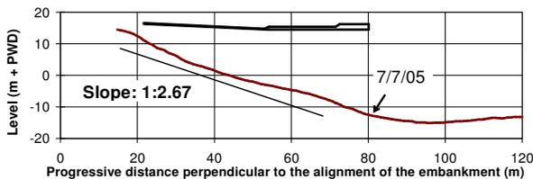
**Fig.10** Typical damaged falling apron with concrete blocks measured at Ghutail FAP 21/22<sup>8)</sup>
