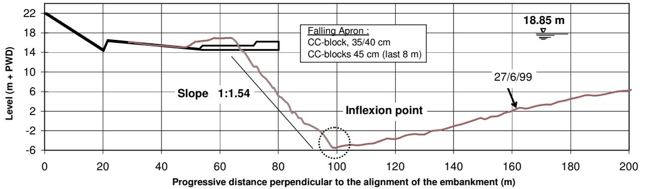
**Fig.7** Cross section with concrete (CC) blocks measured at Bahadurabad FAP 21/22<sup>(8)</sup>. The inflexion point is at the toe and provides the starting point for measuring the slope angles
