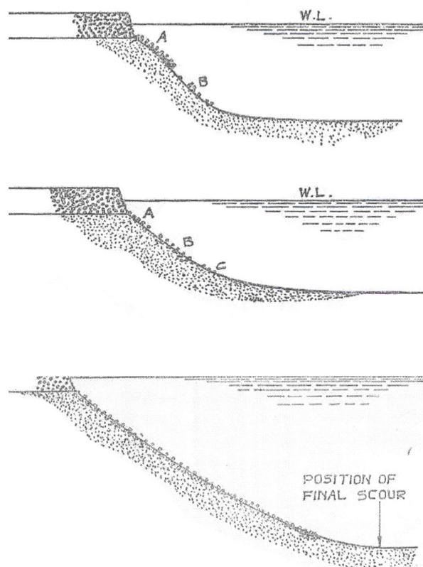
**Fig.3** Inglis<sup>1)</sup>: launching process of falling aprons covering the slope in single layer
