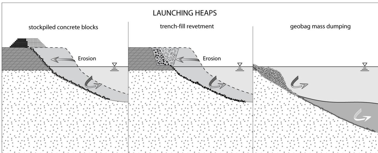
**Fig.2** The principle of launching heaps
