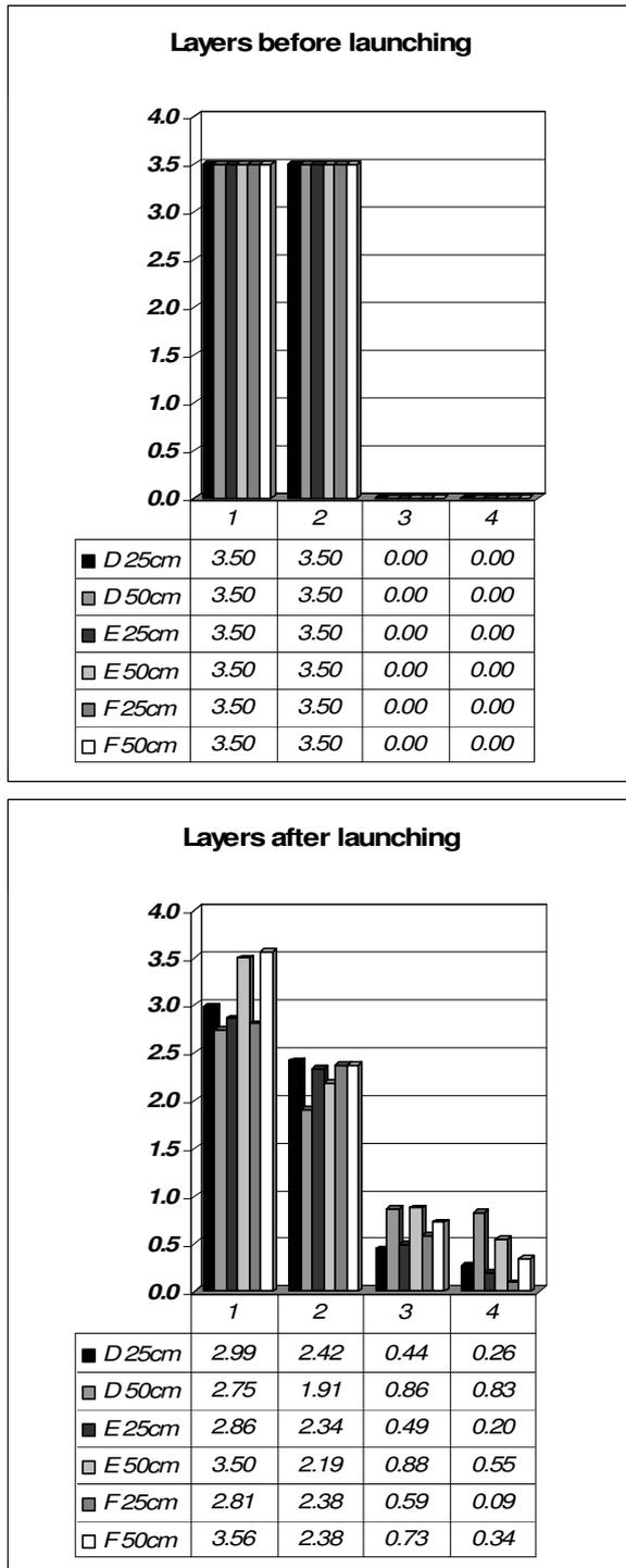
**Fig.4** FAP 21<sup>8)</sup> model tests - layer thickness before and after launching. The concrete blocks were placed along the toe in two parallel segments named 1 and 2 and launched down the slope after scouring. Here they were counted again in two segments named 3 and 4.
